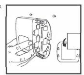
6. With the contacts of the wire harness connector facing you, plug the 6-pin connector end of the Wire Harness into the bottom of the Control Panel.
